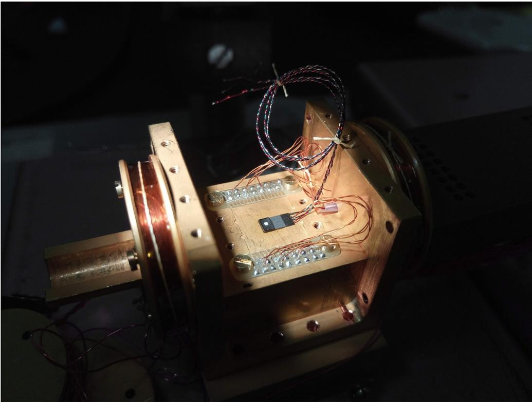
**Figure 3:** The 2Dex Hall sensor mounted in the box for testing. One of the superconducting coils can be seen on the left side of the picture. The Hall sensor is mounted to detect magnetic fields in the y direction.
