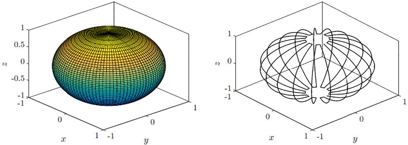
**Figure 5:** Left — surface of the sphere is split into sections of equal area. Right — The path of the scan where the azimuthal angle is fixed as the polar angle is scanned over an arc on the sphere, repeating until the entire sphere is covered.
