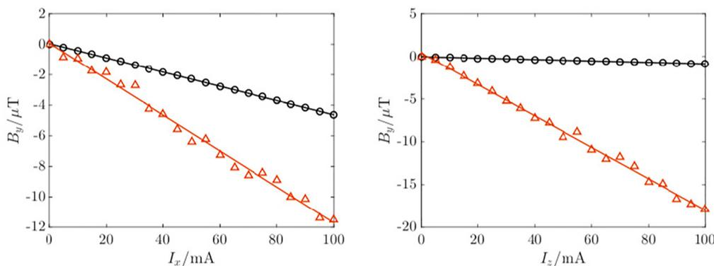
**Figure 4:** The magnetic field in the y direction, measured as a function of current through each coil pair not orientated in the same (y) direction as the Hall probe. The black points show data using the 2Dex Hall sensor; the red triangles show data from the InAs Hall sensor. Left: the response of the sensors when the current in the x coil pair is swept. Right: the response of the sensors when the current in the z coil pair is swept.
