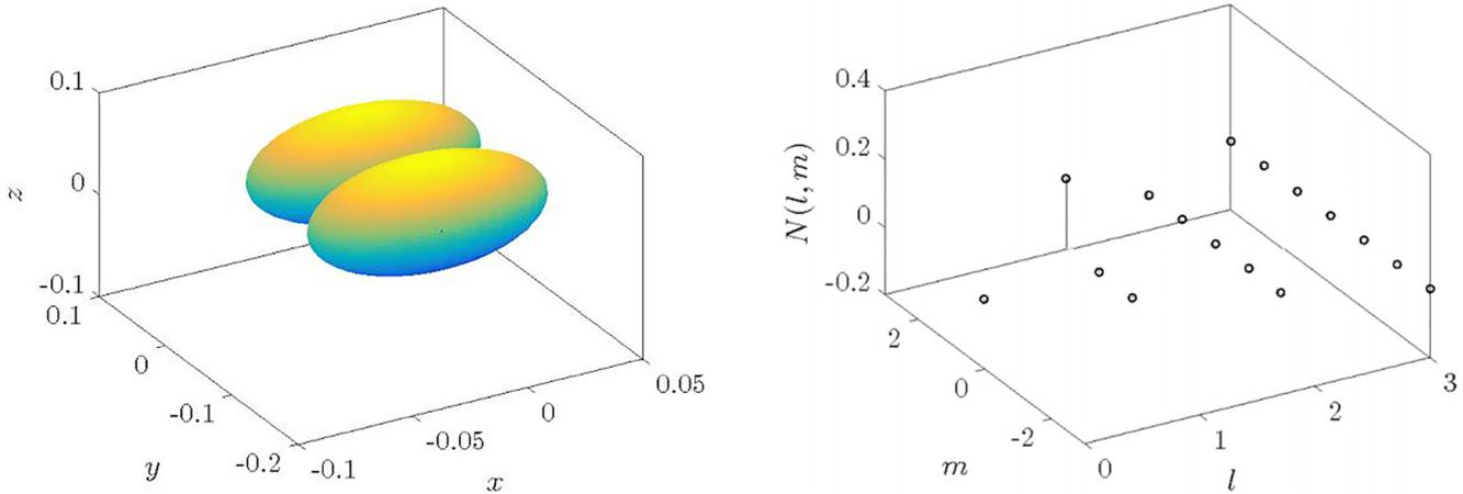
**Figure 6:** (Left) The directional response of the 2Dex Hall sensor to a field of 0.1 mT, expressed using a spherical harmonic basis. (Right) The magnitude of each spherical harmonic component in the directional response.
